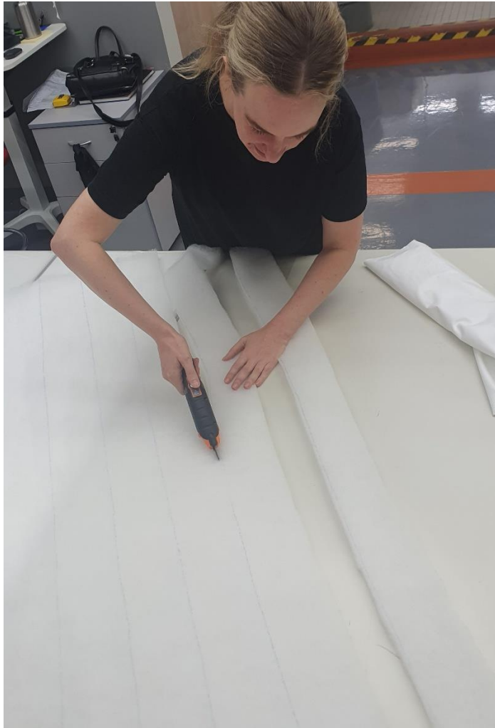
Cutting Dacron using electric scissors
